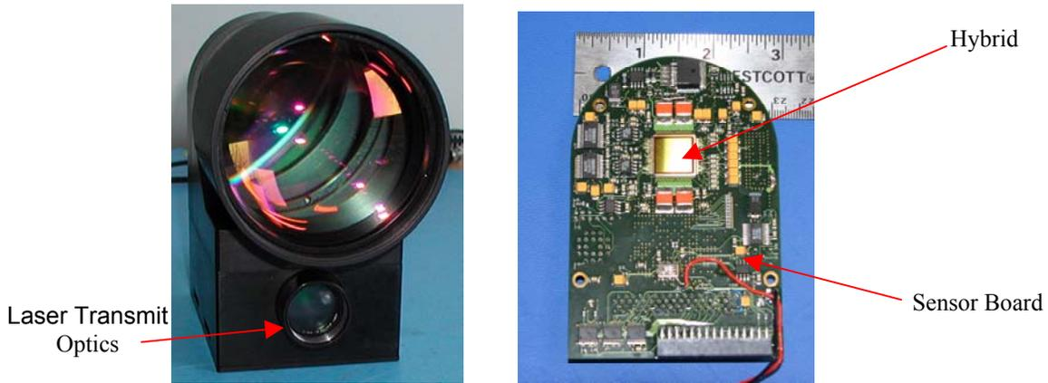
Figure 1. Handheld ASC 3-D Flash Ladar Camera Showing FPA and Associated Electronics as well as ASC Designed Optics. Right hand side (RHS) is the camera sensor board and the Left Hand Side (LHS) shows the laptop-operated camera
