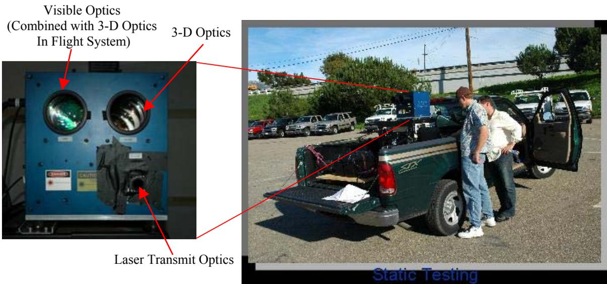
Figure 2. Flight Test System in Static Vehicle Test Configuration. The goal of this system development project is a UAV-based topographical mapping system with the capability of 350  $\text{km}^2/\text{hr}$ , a volume less than 1  $\text{ft}^3$  and a total weight including GPS and INS less than 50 lbs.
