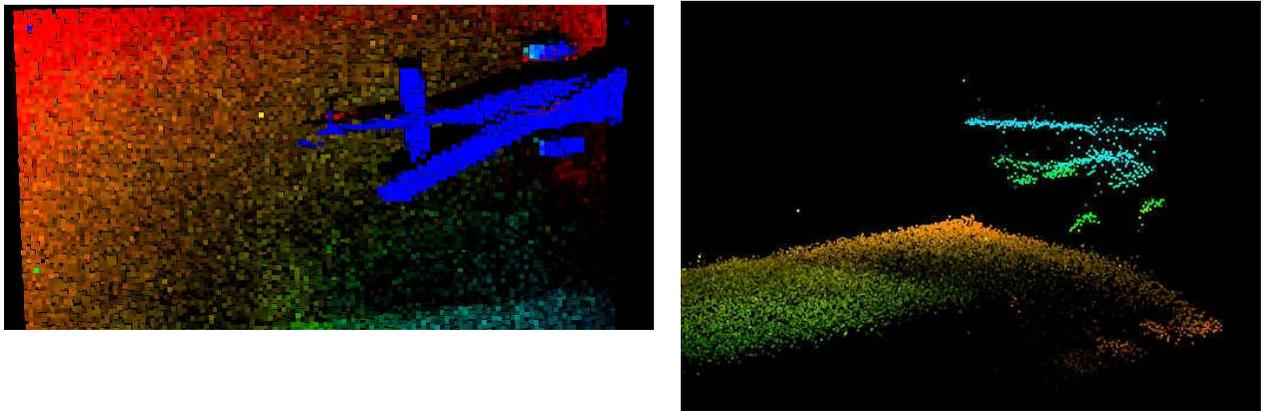
Figure 4. Two Orientations of the Same Helicopter 3-D Image at 1300 ft. Left hand side is down looking and right hand side is a front looking, rotated 3-D image. Note the shape of the rotor blade is captured by the speed-of -light system and that rotation of the 3-D image dramatically increases the capability for object recognition.
