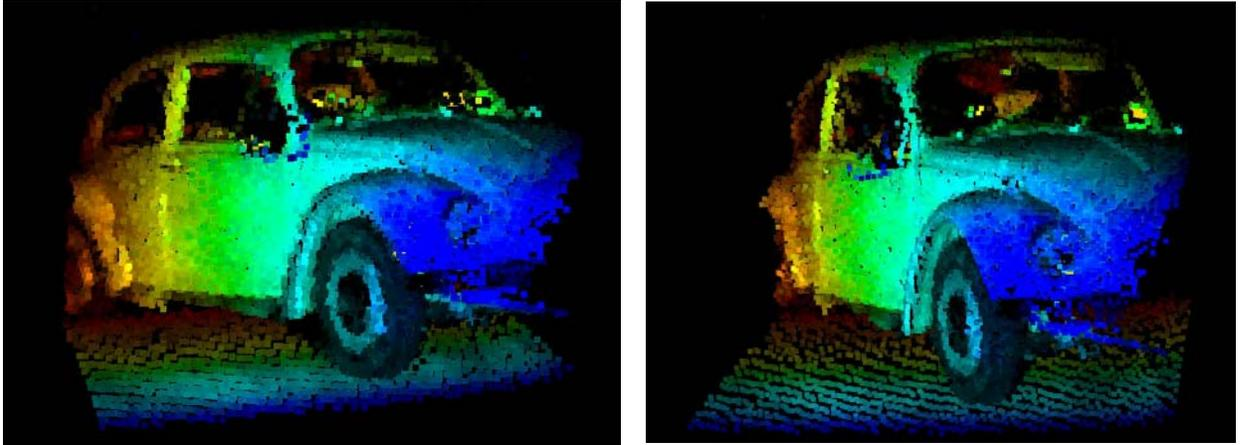
Figure 3. Two Orientations of the Same Single-Laser-Pulse 128 x 128 3-D image. Data was processed using the ASC range algorithm only and so is essentially a raw-data image. Color-coded for depth. Although a raw image, the vehicle type is clear.
