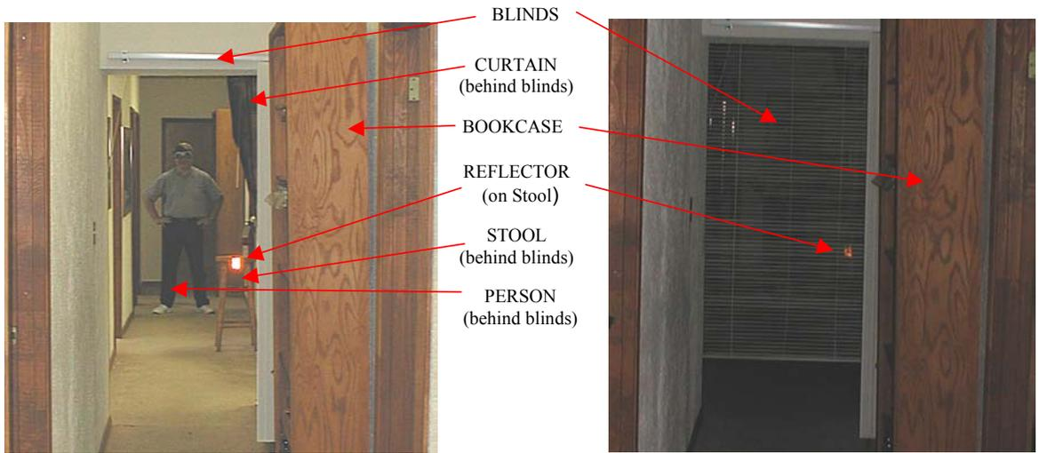
Figure 7. 2-D Pictures of Camouflage Penetration Experiment. (LHS) Blinds pulled up to show person and stool behind blinds. (RHS) Blinds down and closed 50%. Stool and person are totally obscured in the 2-D image. Some light from the reflector on the stool appears in the 2-D image.
