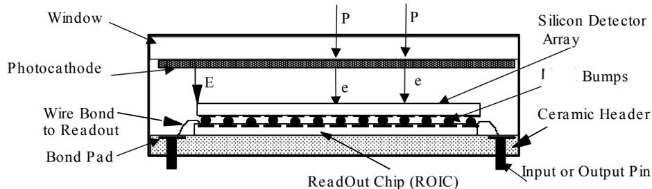
Figure 3. Electron Bombarded (EB) Image Tube 3-D FPA
