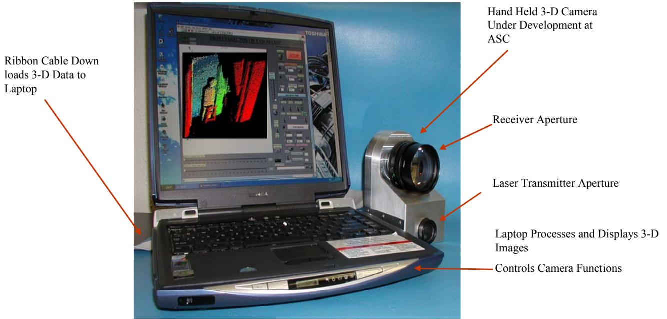
Figure 1. Representative 3-D Flash Ladar Imaging System
