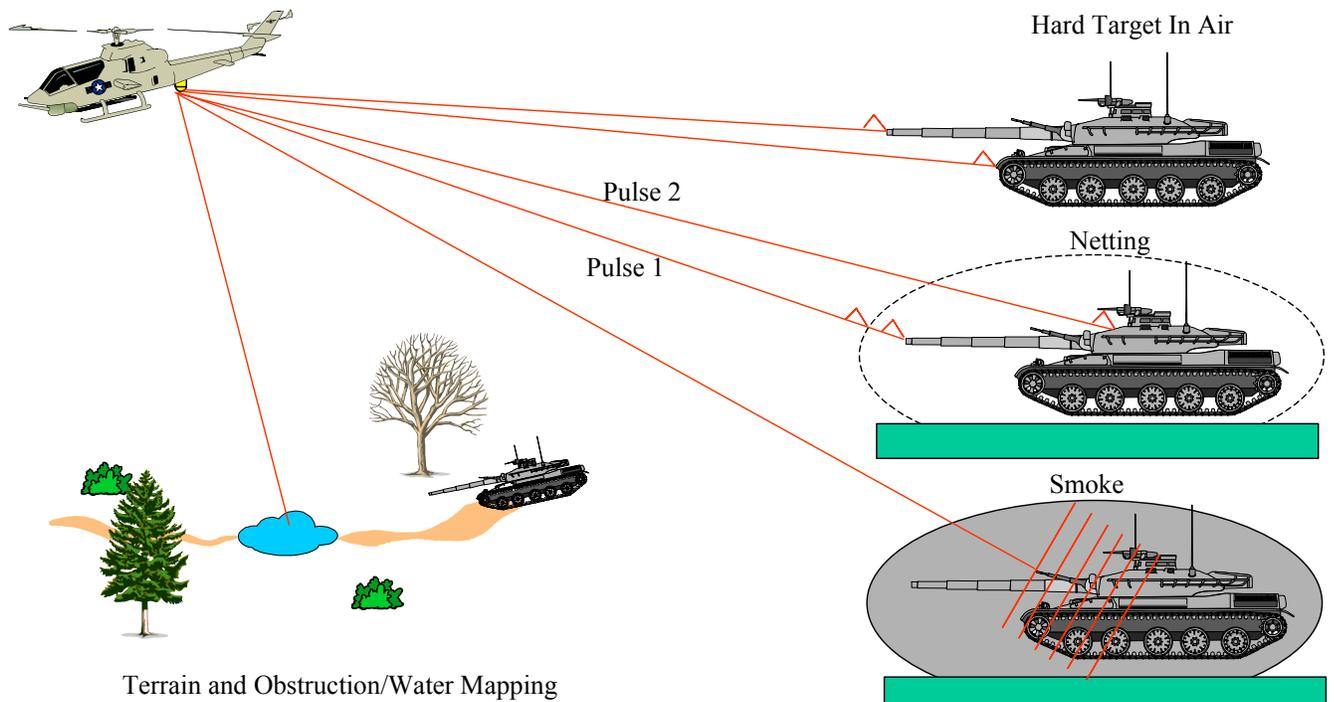
Figure 4. Function of AVDAR ROIC: hard target 3-D imaging, 3-D imaging through camouflage, 3-D imaging through smoke and 3-D imaging through water.
